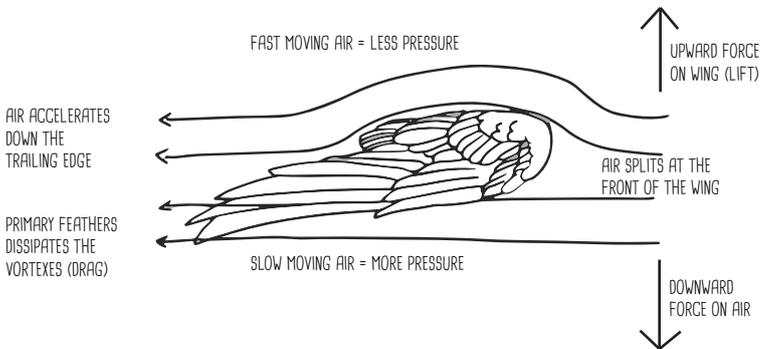
The wings of vultures are broad and long with a slight curve at the top. This gives the top part more surface area than the bottom. Air will move faster over the bigger surface area than the smaller surface area which reduces the air pressure and creates lift.
